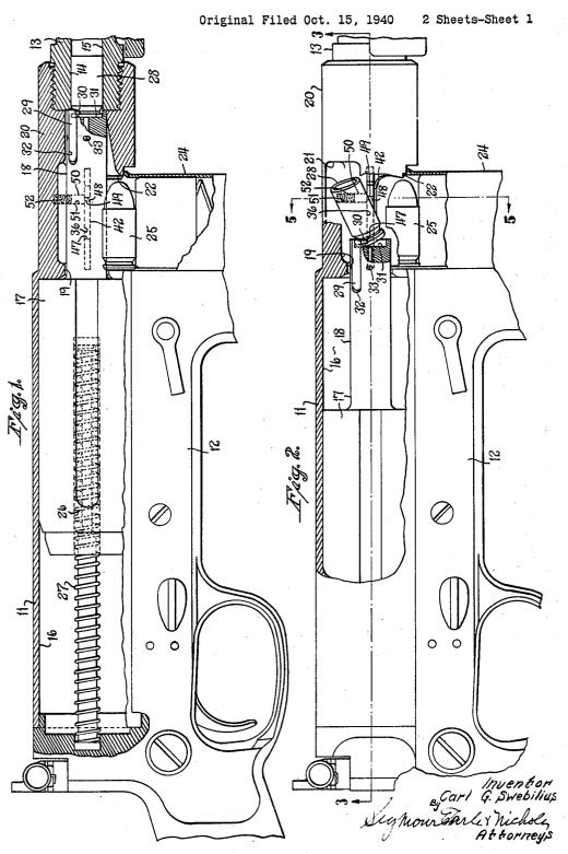
CARTRIDGE-EJECTING MEANS FOR FIREARMS
